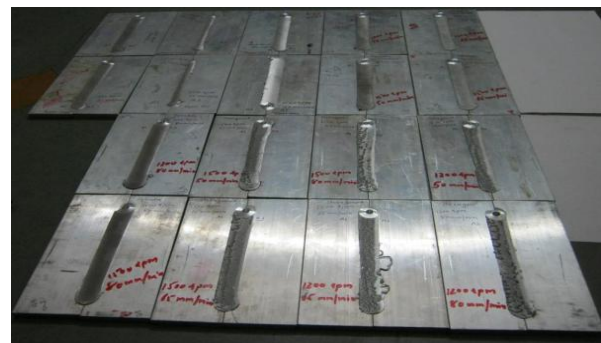
Fig: -5 FSW Joints of AA6082-T6
