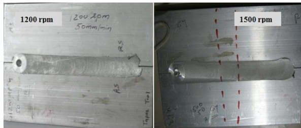
Fig: -7 Welded Specimen at 1200 and 1500 rpm
