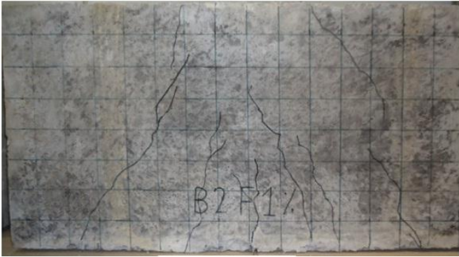
Fig 9 Crack Pattern of beam D40 AR80 [F1%]
