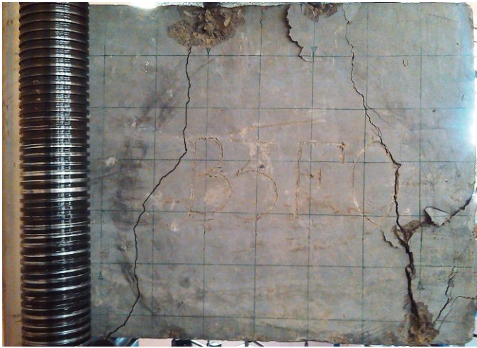
Fig 22 Crack Pattern of beam D60 NRC [F0%]
