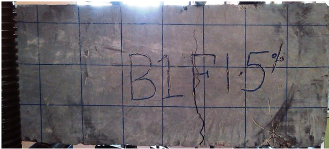
Fig 16 Crack Pattern of beam D30 AR50 [F1.5%]
