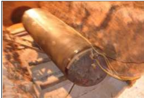
Fig. 11 Test Pressure Vessel
