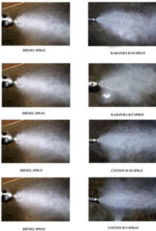
Fig.3. photograph of spray comparison for diesel and different biodiesel blends
