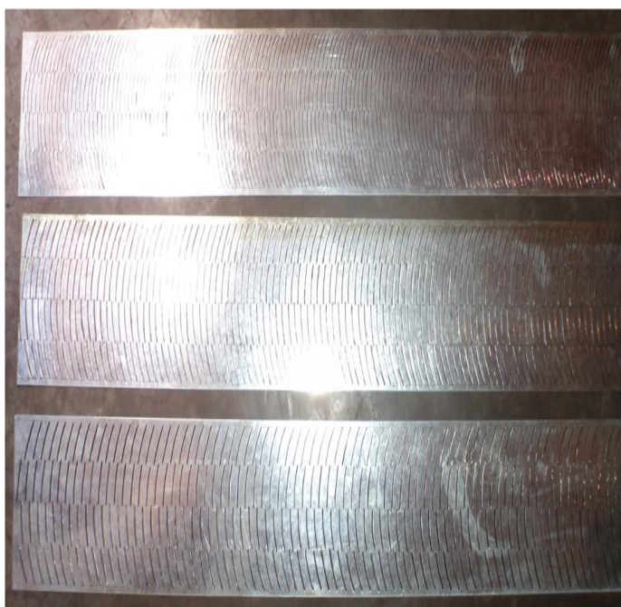
Fig.3 Actual photograph of absorber plate of different pitches
