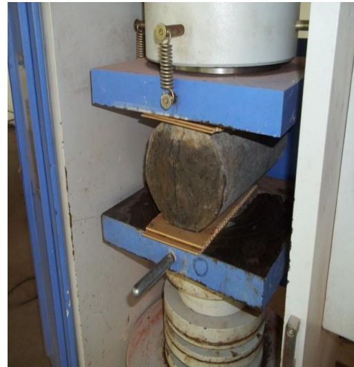
Fig 3.splitting tensile strength test
