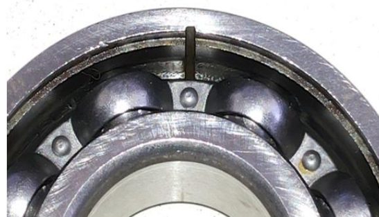
Fig. 3 A 1 x 0.5 mm defect on the Outer Race
