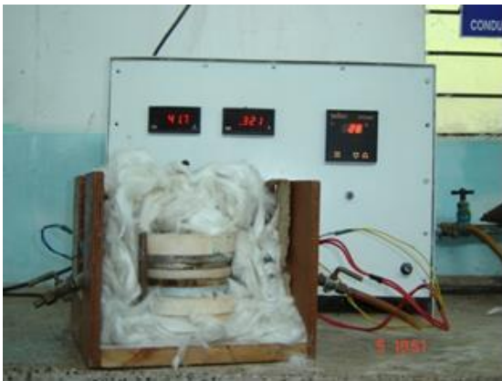
Fig 2. Thermal conductivity test setup
