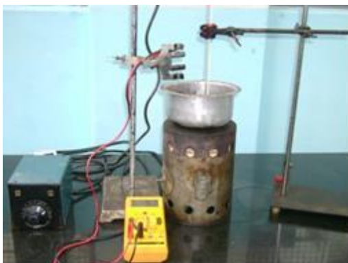
Fig 4. Specific heat test set up
