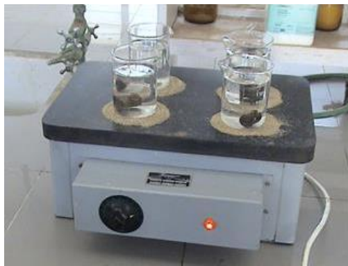
Fig 8. Test set up of Hot Boiling Test
