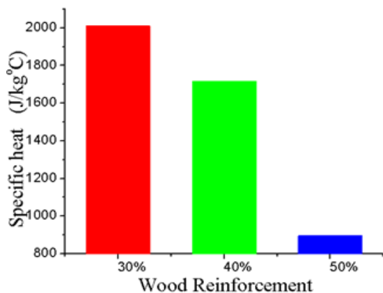
Fig 12. Specific heat v/s reinforcement percentage
