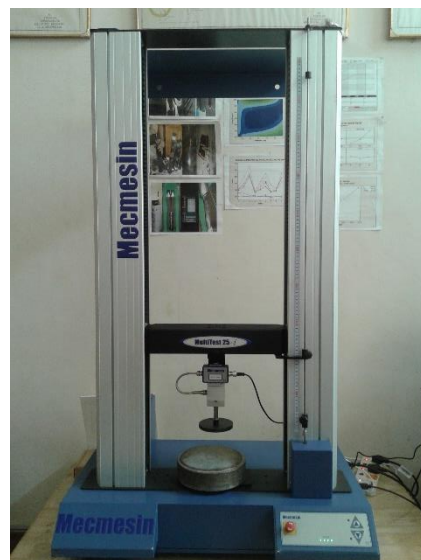
Fig 4: MultiTest 25-i Nano Universal Testing Machine (Funded by VGST, Bangalore)
