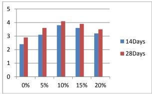
Chat 2 split tensile strength % PET replacement %Steel fibre
