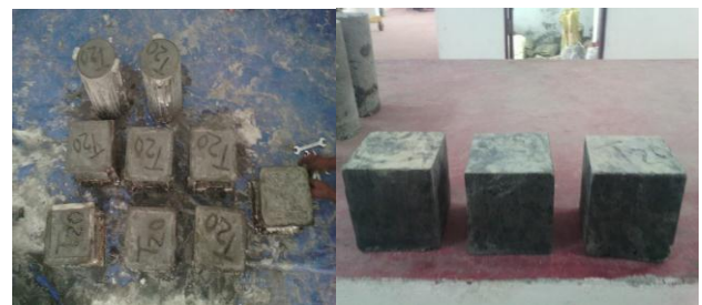
Fig. 4.Casting of cube specimens
