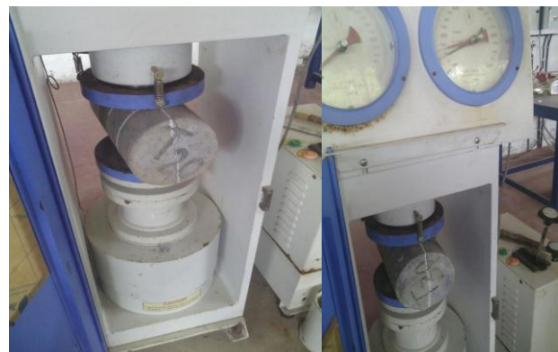
Fig. 7. Split tensile strength test
