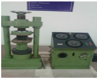
Fig. 4. Testing of cube specimens
