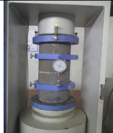
Fig 9. Modulus of elasticity test using extensometer
