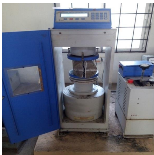
Fig-4 : split tensile strength test
