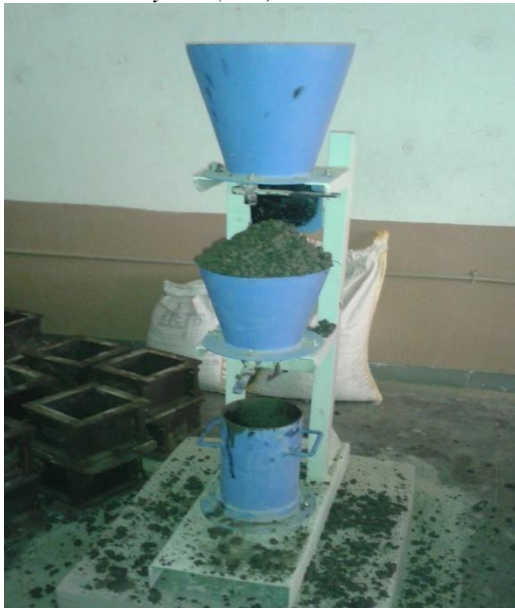
Fig- 7 : Workability test
