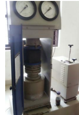
Fig.3. Compressive strength testing machine
