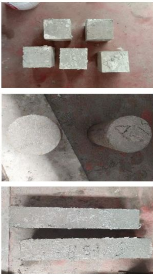
Figure 2: Casting of specimens
