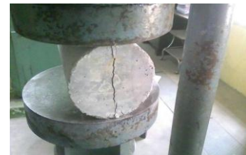
Fig.2 Testing of cylinder specimen for Split tensile strength
