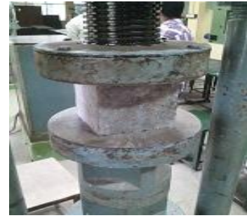
Fig.1 Compressive strength test of concrete cube specimen
