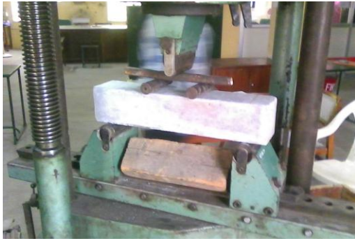
Fig.3 Flexural strength test of prism specimen
