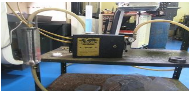
Figure 2: Photo graphic view of external MQL setup
