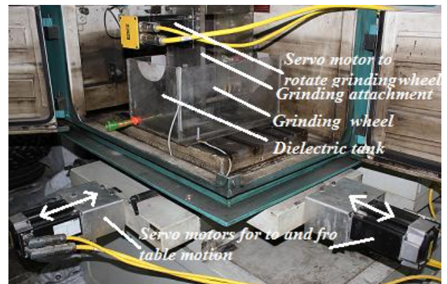
Figure 2 Attached EDG setup on EDM machine
