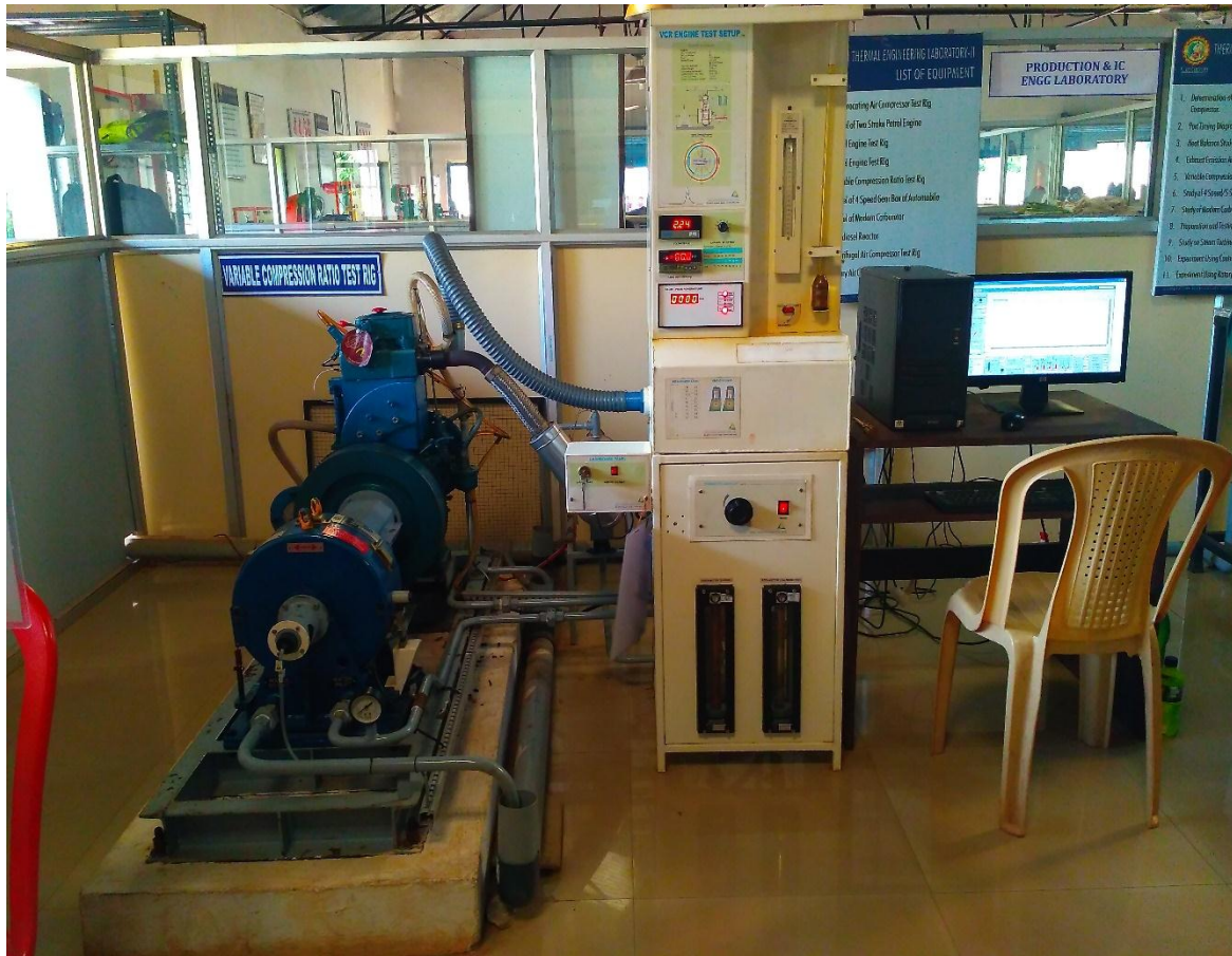
Fig.4.4. Experimental Setup of Computerised C.I Engine
