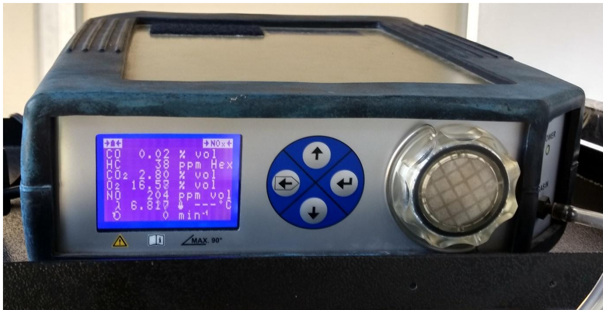
Fig.4.3. Five Gas Analyser with Display
