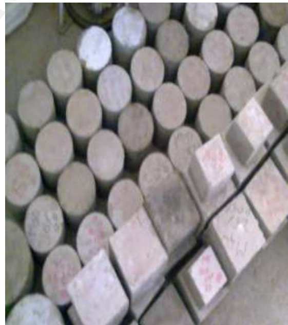
Fig-4: The concrete specimens are cured in room temperature
