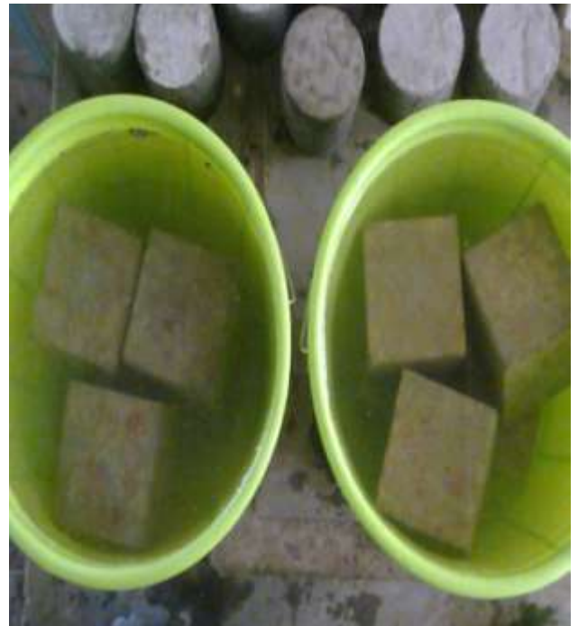
Fig-2: The cubes were immersed in the Na 2 SO 4 solution
