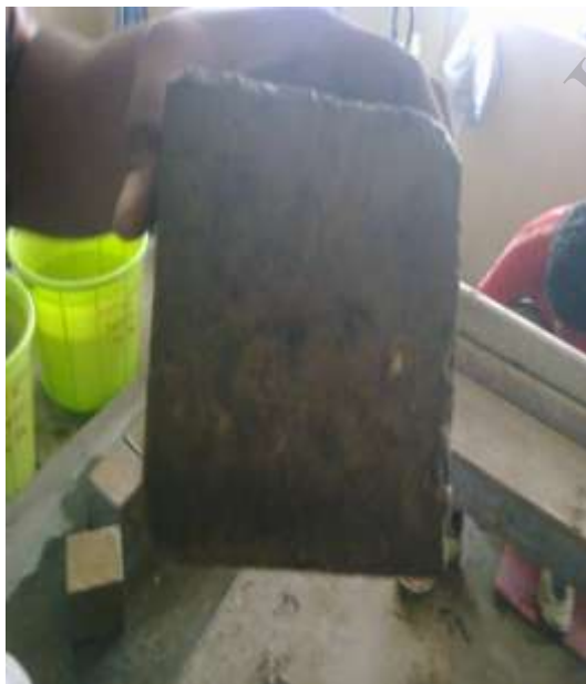
Fig-3: The deteriorated concrete specimen On the 3 rd day
