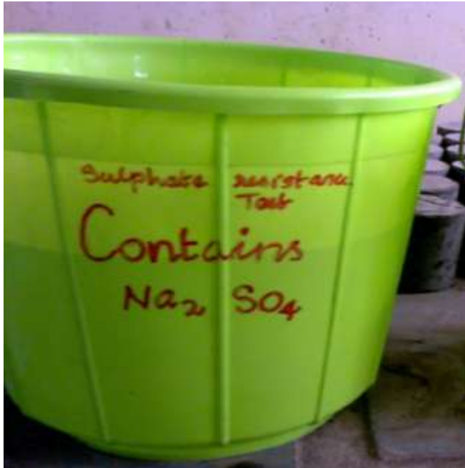
Fig-1: The container contains Na 2 SO 4 solution
