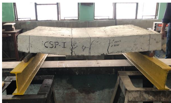
Fig. 5: Flexural Cracks formation of CSP – I
