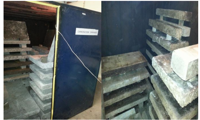
Fig 2:Slabs in carbonation chamber. Fig3: Carbonated slabs.
