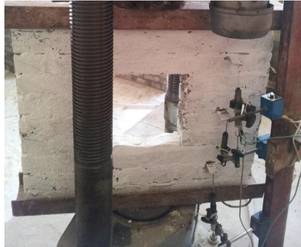
Fig. 12 Wall deformations measured with LVDT
