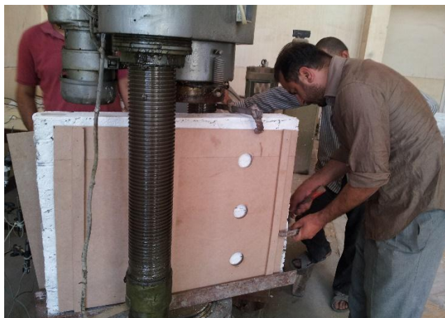
Fig.11 Carrying wall on testing machine by wood panels
