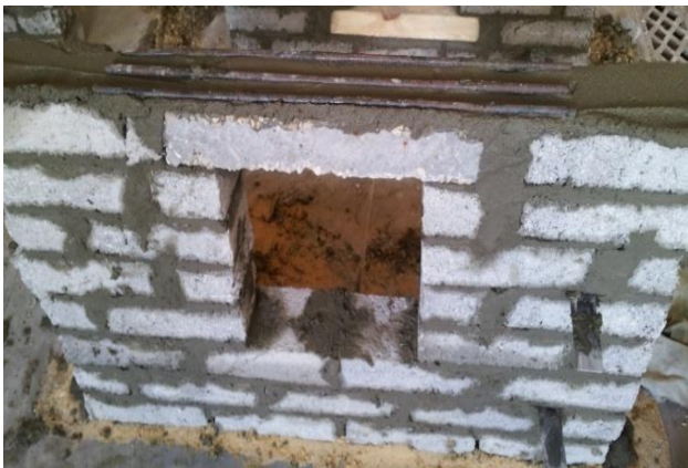
Fig. 4. Strengthening brick walls with opening using 3Ø8 steel bars embedded into bed joint mortar above lintel only with length (L1 = 50 cm)
