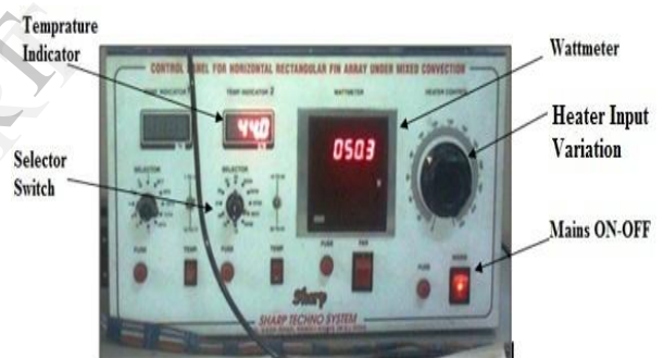
Fig.3. Photograph of Digital Wattmeter and Digital Temperature Indicator
