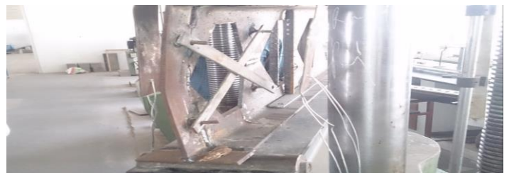
FIGURE 11 shows the web buckling of IC300 WDS&WVS
