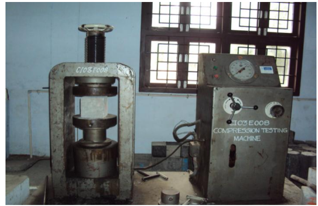
Figure 3. Experimental setup of compression test
