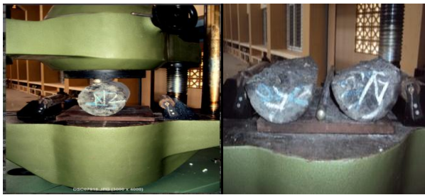
Figure 5. Experimental setup of Split Tensile
