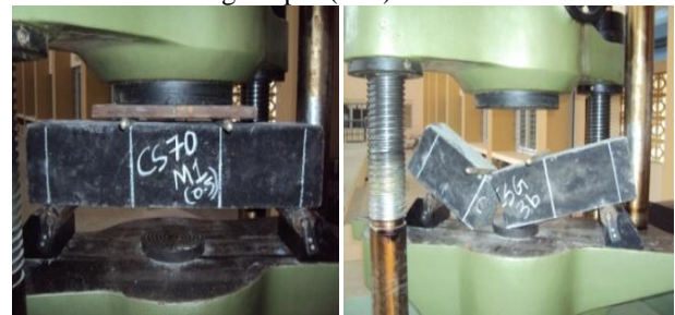
Figure 7. Experimental Setup of Flexural Test
