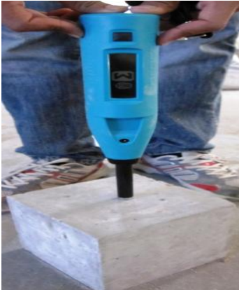
Figure – 2 Rebound Hammer test
