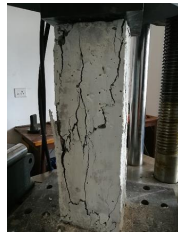
Fig 7. Failure pattern of control specimen
