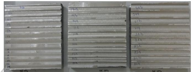
Figure 5: CNC End milled LM6 Al/SiC workpieces at different SiC%
