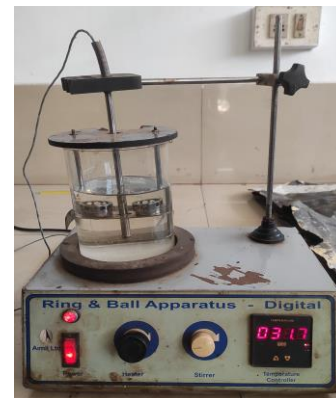
Fig.2. Ring and ball apparatus
