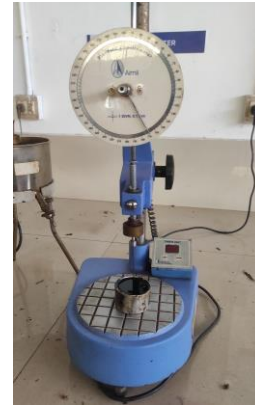
Fig.1. Penetrometer B. Softening Point Test
