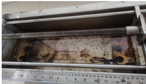
Fig.4. Ductility test apparatus
