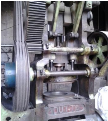
Fig.3: Mechanical press used in deep drawing process
