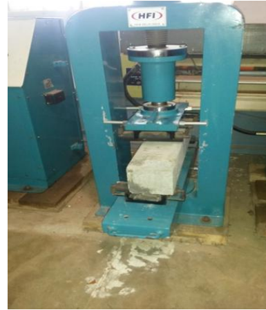
Fig 3 .Flexural Strength testing
