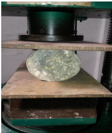
Fig 2 Split Tensile testing
