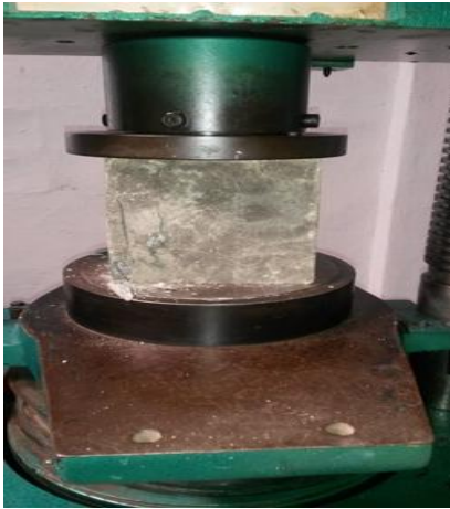
Fig 1. Testing of Compressive strength
