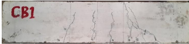
Plate 2.failure pattern of conventional concrete beam
