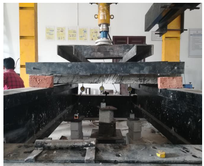
Fig 4. Test set up, Loading frame (50Ton capacity), used for testing
