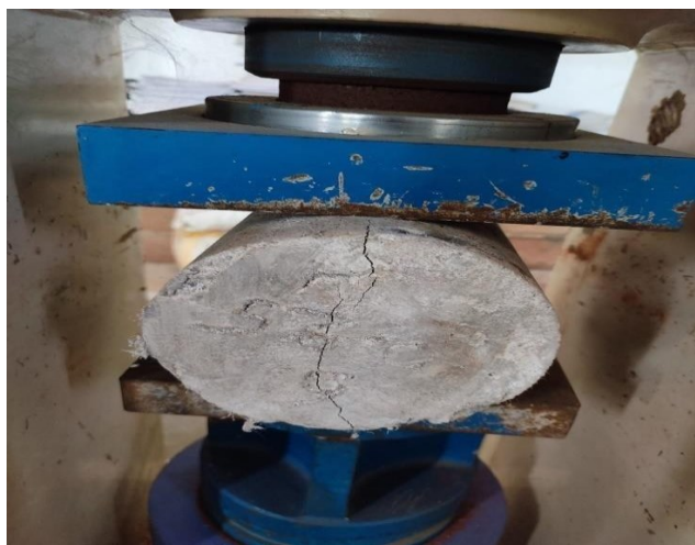
Figure 3: Cylinder Under Split Tensile Testing Machine
