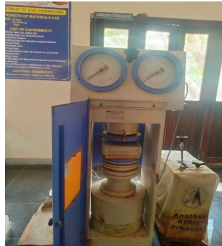
Figure 1: Cube Under Compression Testing Machine
