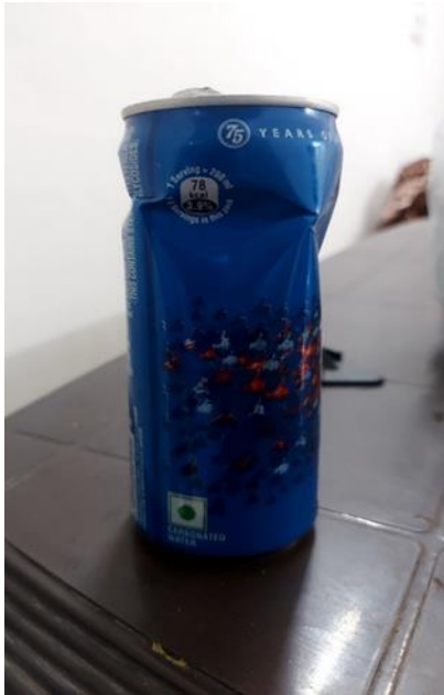
Fig. 8. Buckling of test specimen with full of liquid
