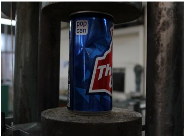
Fig. 2 (Test specimen I), (a) & (b) D.S. buckling observed around 3 cm from top
