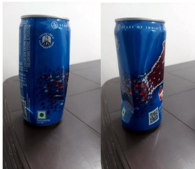
Fig. 5 (a) and (b). series of small Diamond shaped buckling formed along with twisting and axial bending due to foot loading
