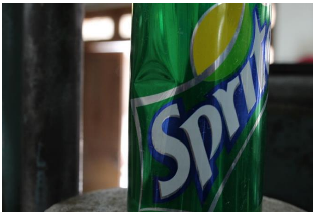
Fig. 3 (Test specimen II), D.S. buckling observed around 5 cm from top
