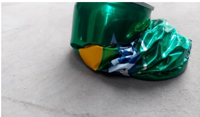
Fig. 5 (a) and (b). series of small Diamond shaped buckling formed along with twisting and axial bending due to foot loading
