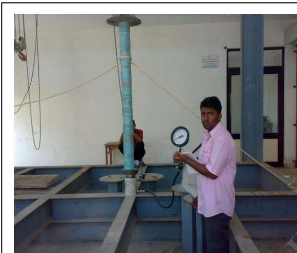
Photo.1 Compression test set-up for long column
