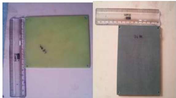
Figure 13: Dielectric superstrate ( \epsilon_{r2} ) is 3.2 and superstrate materials ( \epsilon_{r2} ) is 4.8
