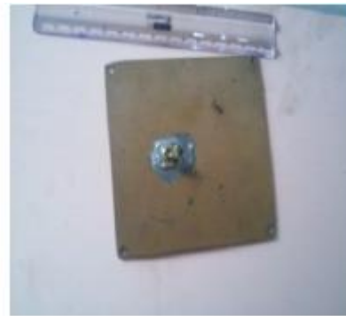
Figure 11: Fabricated Porto type square patch with feed point location
