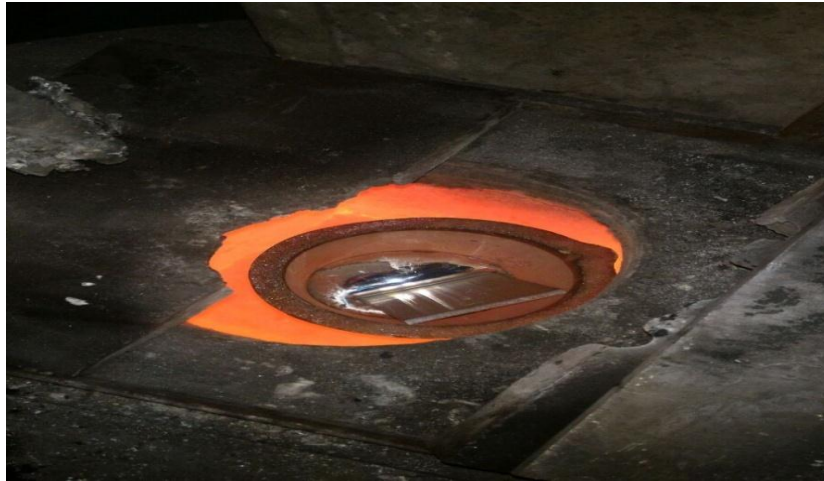
Fig 2.5: Aluminium 2024 sinking and melting inside the crucible inside the furnace.
