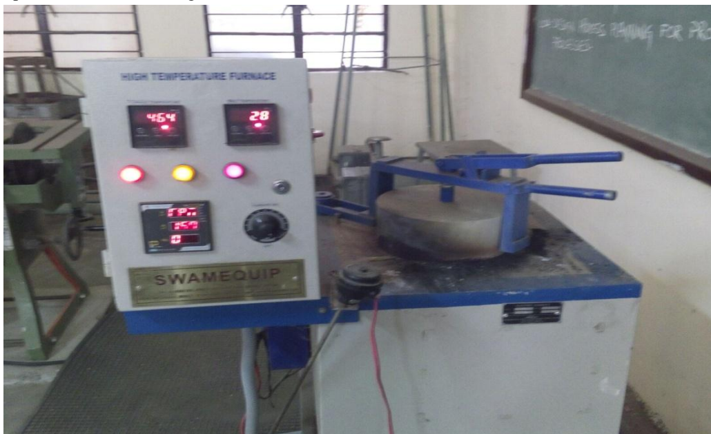
Fig 2.3: Pre- heating furnace
