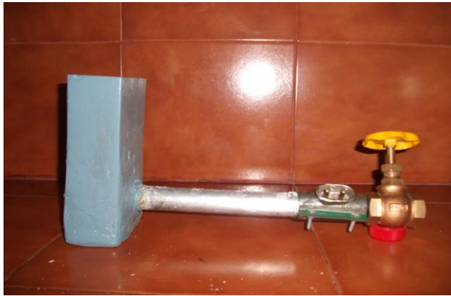
Fig.1 (a) Fabricated Heat Pipe with valve
