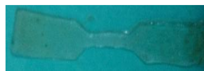
Fig 5: ASTM D638 Type PVP +KI+AlN nano composite sample
