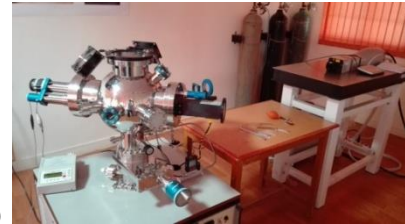
Figure 1(a) Schematic working of Pulsed Laser Deposition (b) ZnO pellet placed in the target and (c) Instrument setup: Pulsed Laser Deposition System – 12 – 100 (Excel Instruments) and Solid State Pulsed Laser Source (Quantel Laser System – Qsmart 450mJ).
