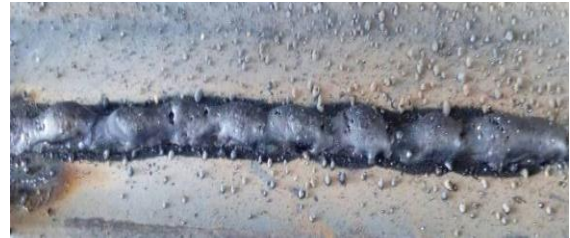
Figure 1.9: Bead on plate performed by the semi-automatic arc welding machine.
