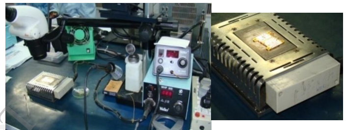
Fig: 5 Substrate Attachment on Kovar Carrier plate
