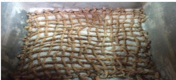
Fig. 1. Geotextile reinforcement as grid pattern of 20 mm × 20 mm
