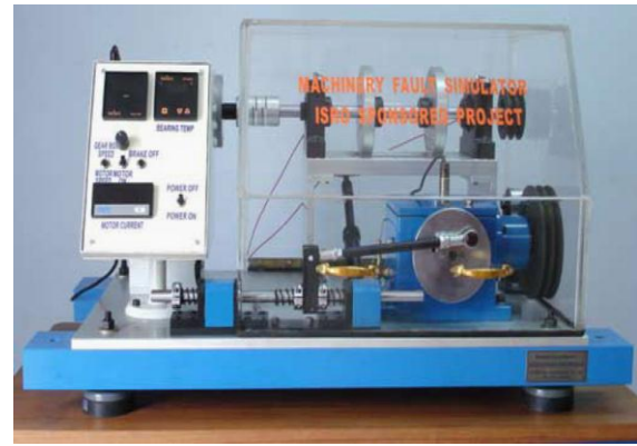
Fig. 2. Machine fault simulator setup.
