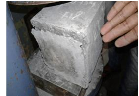
Fig 4(b). Failure of cube
