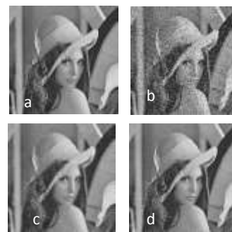
Fig.8 Subjective performance illustration of the proposed filtering technique compared with existing technique: (a) Original Lena image, (b) Lena image Corrupted by 10% impulse noise and gaussian noise with zero mean and \sigma^2=200 , (c) Restored by multiple noise elimination, (d) Restored by the proposed filter
