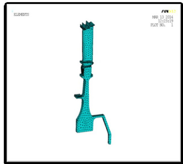
Fig.3 Meshed FE model of single cut section with disc.
