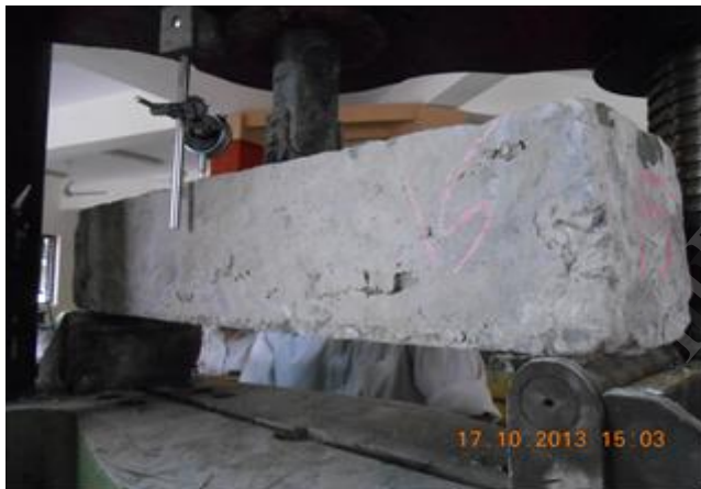
Figure 4 (Pre-retrofitting flexural loading.)
