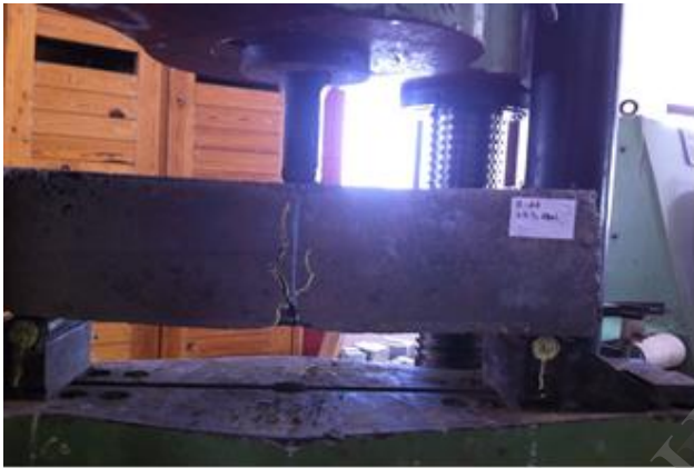
Figure 6. (Flexural testing of beams.)
