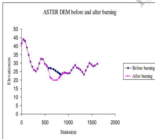
Figure 10.1. DEM Before and After Burning
